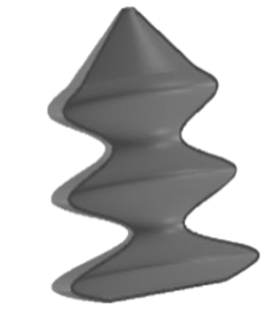
Mathematical design inspired by exponential decay for natural tapering of arm.
